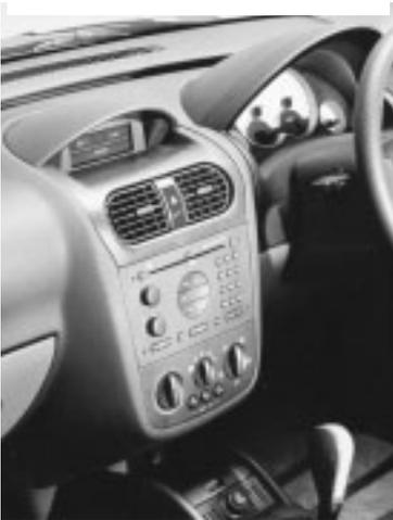
The MFD is positioned carefully within the driver's forward field of vision so that information can be read at a glance. Models such as the Astra, Omega and Vectra even incorporate information from the trip computer on the MFD.
