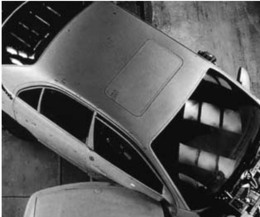
Prototype Omegas were tested in a wide range of frontal, side and offset impacts.
