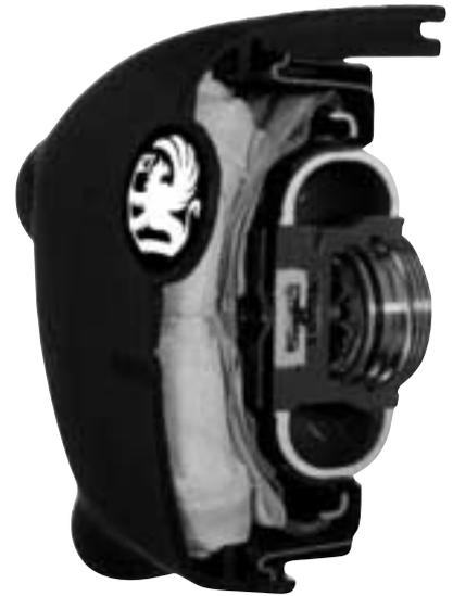
A sectioned view of the hybrid airbag
