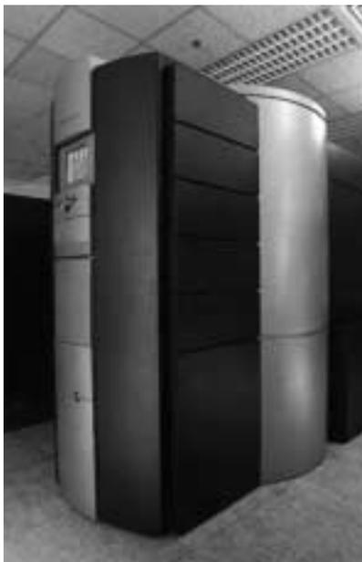
Today, the Centre has the latest generation Cray C90 which performs an astonishing 4 billion operations per second. This degree of sophistication allows designers to develop passive and active safety features with the utmost reliability and predictability.
