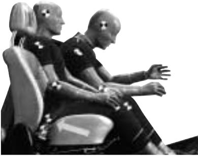
This test demonstrates the effectiveness of three-point seat belts, Vauxhall's Body-Lock system and anti-submarine seats.
