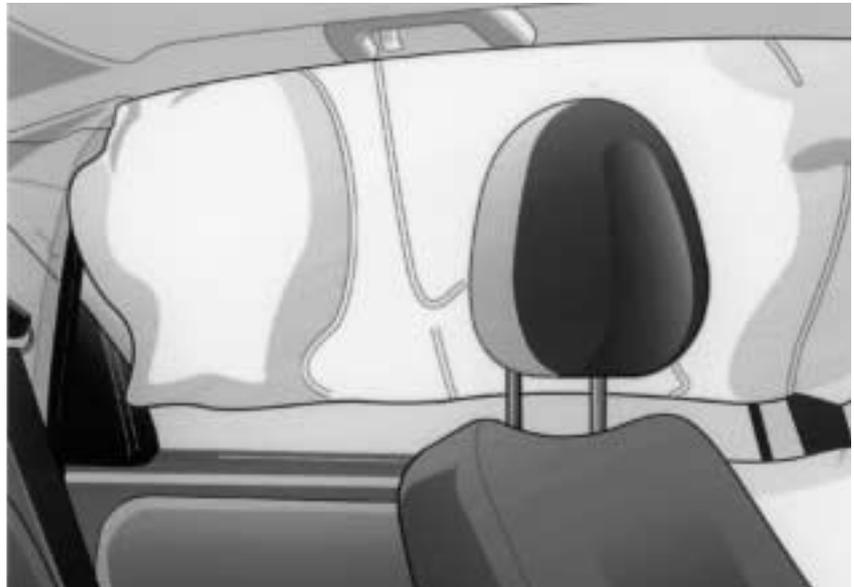
Diagram shows the curtain airbag system fully deployed.
