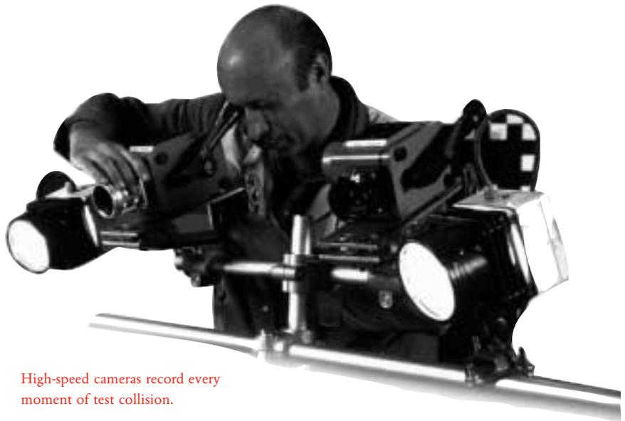
**High-speed cameras record every moment of test collision.**
