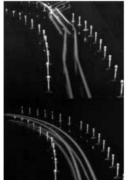
The lower picture clearly shows the advantages of ABS braking when cornering.
