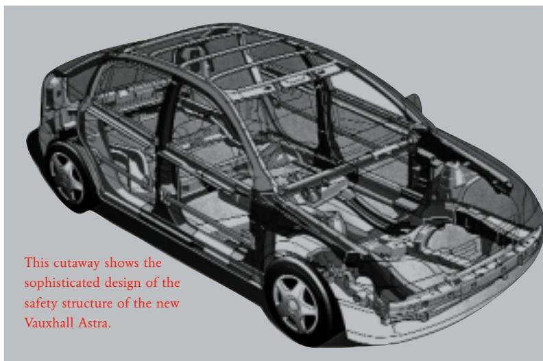
This cutaway shows the sophisticated design of the safety structure of the new Vauxhall Astra.
