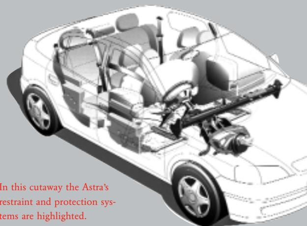
In this cutaway the Astra's restraint and protection systems are highlighted.
