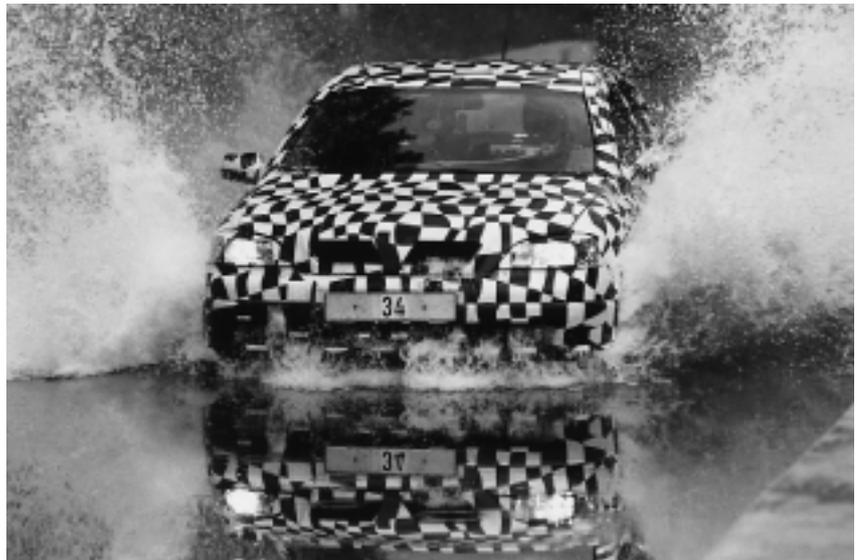
This dramatic water test was conducted to establish the straight-line stability of the prototype Vauxhall Astra passing through heavy surface water. This test simulates conditions far worse than most drivers would ever experience.
